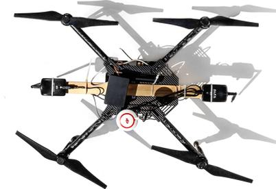
**Figure 3.** Our UAS, a DJI Matrice 100 quad-copter.
